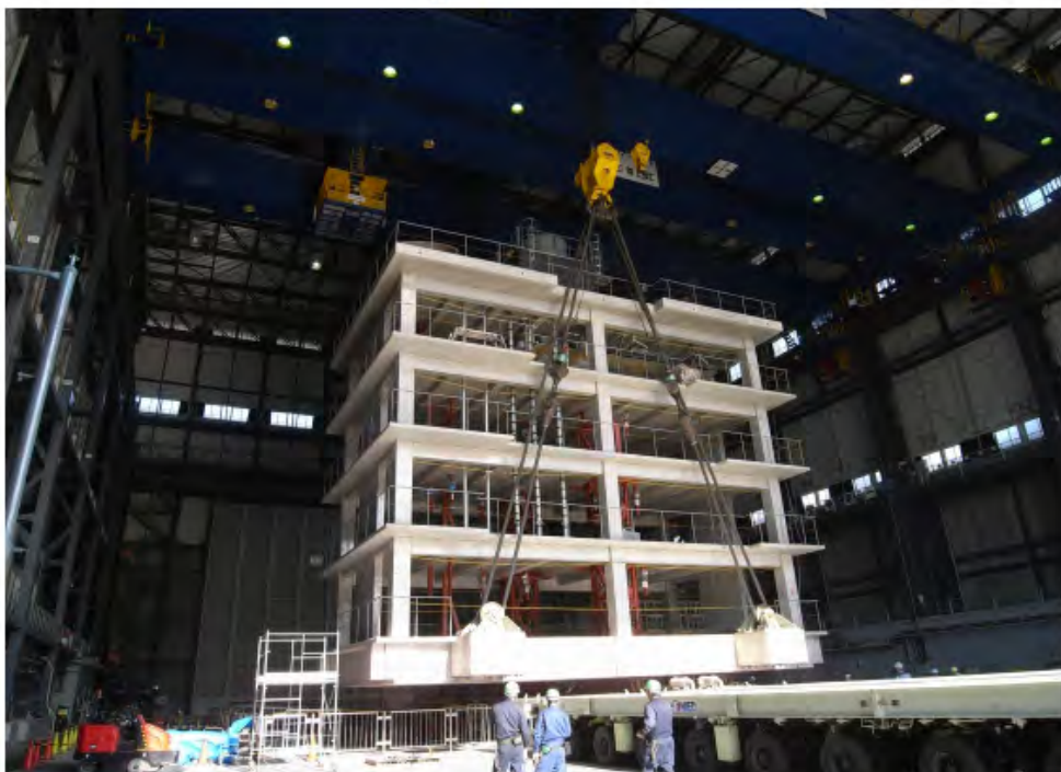
Photo 2. Specimen Hanging on Cranes
