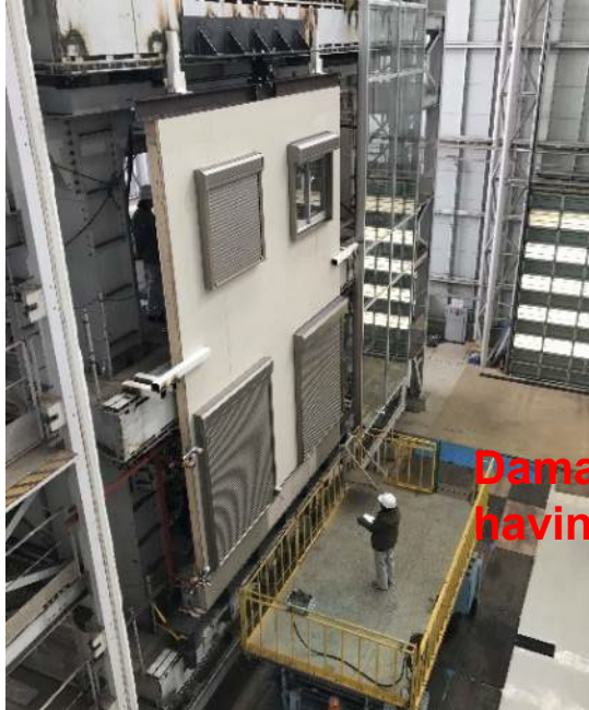
Preliminary exterior frame test (Curtain wall company FUJI SASH)
