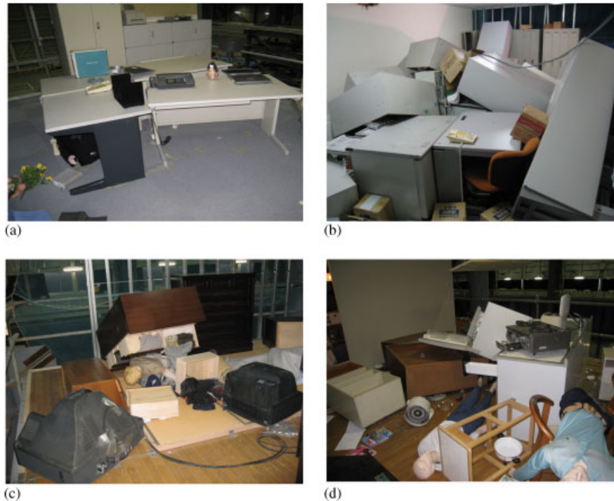
Figure 16. Damage to furniture after shaking: (a) office where furniture is clamped; (b) office where furniture is not fixed; (c) living room; and (d) kitchen.
