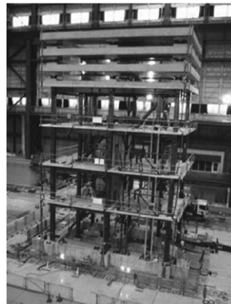
(a) benchmark high-rise steel building on the E-Defense shaking table
