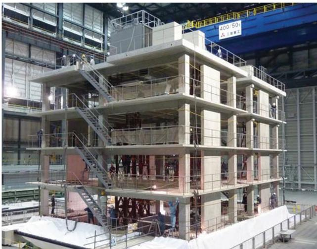
Fig. 2—Reinforced concrete (left) and prestressed concrete (right) specimens on the E-Defense shake table.
