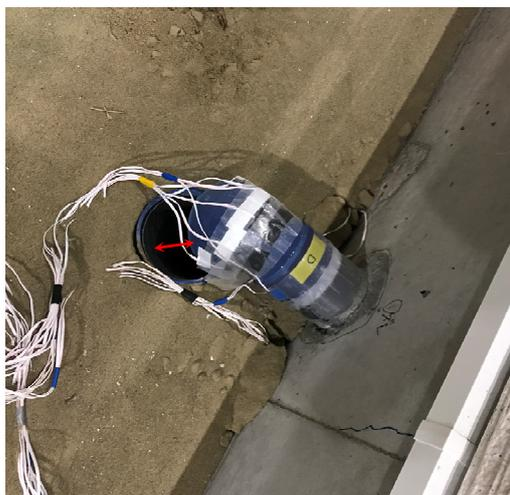
(1) Fractured VP drain pipe
