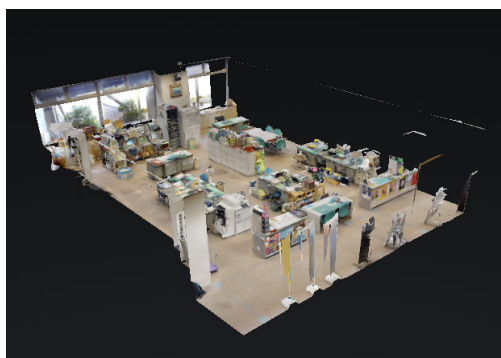
Fig.24 Point Cloud 3D Scan of an office room
