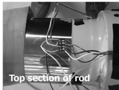
Photo 7 Strain gauges installation on oil damper rod
