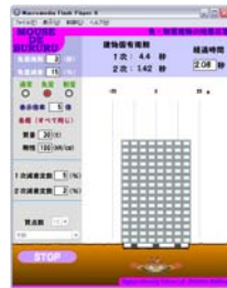
(b) Linear dynamic simulator for multi DOF's system considering base-isolation and vibration control
