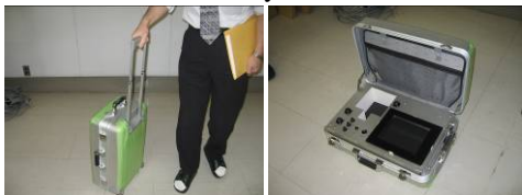
Photo 1 'μ' which is able to identify resonant building by evaluating the period and damping using H/V and the RD method, respectively
