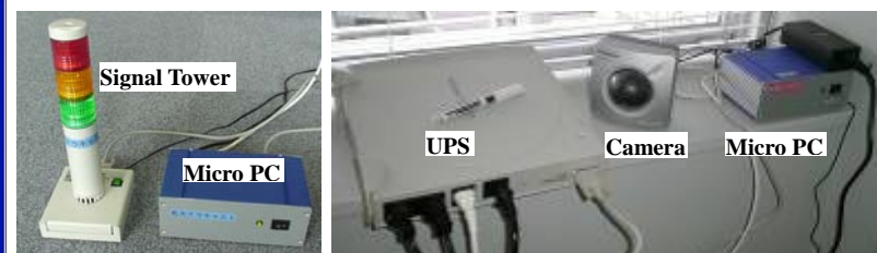
Fig.7 Display and Signal Tower of the Earthquake Alarm System
